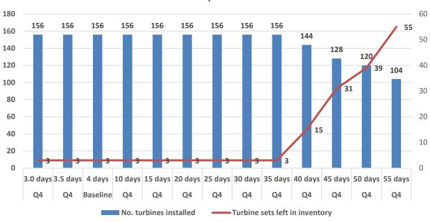
Y1 axis = number of turbines installed, Y2 axis = number of turbine sets remaining in inventory. The test value of 3.5 days matches baseline output option (4 days).
