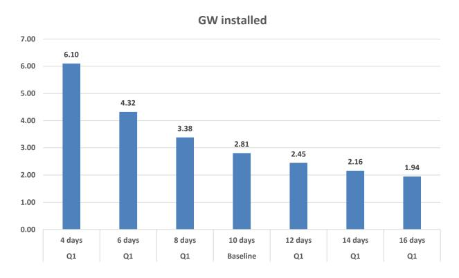
Same observation as for turbines installed, ie the non-linear relationship between resupply ship interarrival time and GW installed is noteworthy.
