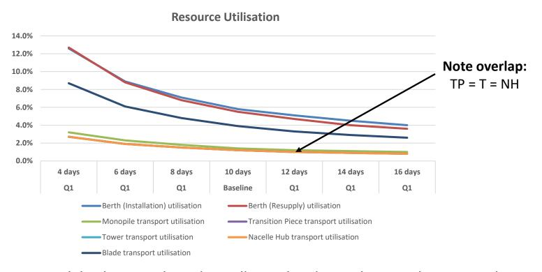
As expected, both resupply and installation berths are busier when resupply interarrival time reduces. And with corresponding unloading and loading events, transport resource utilisations follow a similar pattern.
