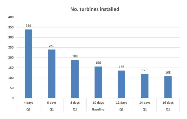
The non-linear relationship between resupply ship interarrival time and number of turbines installed is noteworthy.
